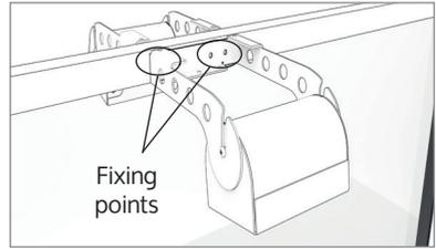
7. Install the power supply close to a power socket outlet using the supplied mounting bracket and fixing screws.
