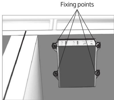
6. Install the overhead loudspeakers:
