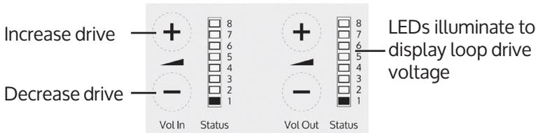
The drive level should be adjusted so the red LED 8 is illuminated only when there are peaks in the speech volume.
