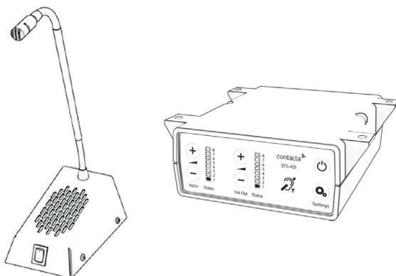
1. Place the Staff Loudspeaker Unit on the staff side of the counter top, ensuring that it does not cause an obstruction and is as close to staff as possible.
