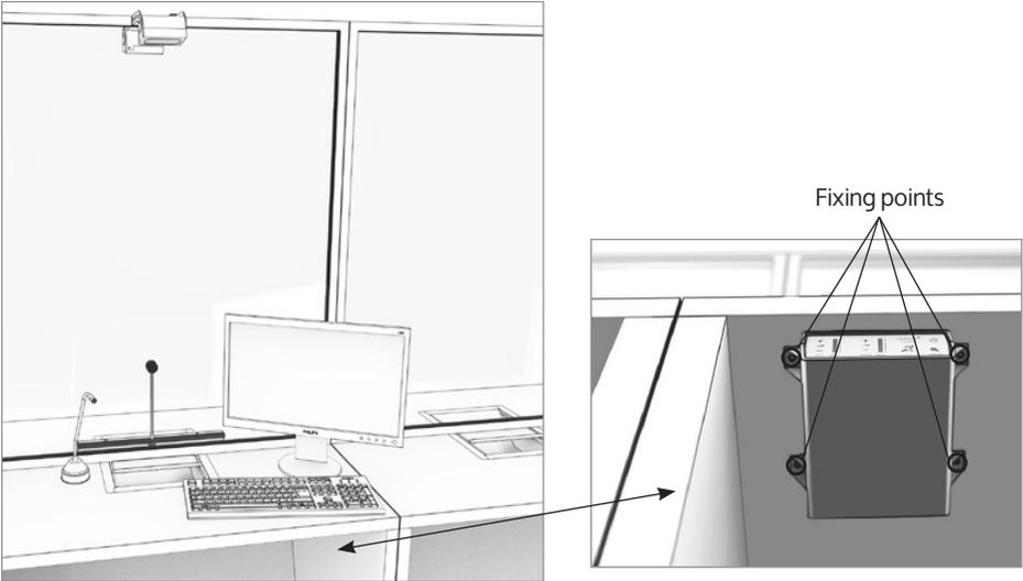
1. Place the staff microphone on the staff side of the counter top, ensuring that it does not cause an obstruction and is as close to staff as possible.
